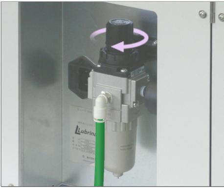
3. After draining the regulator, turn the dial back to adjust the pressure.
