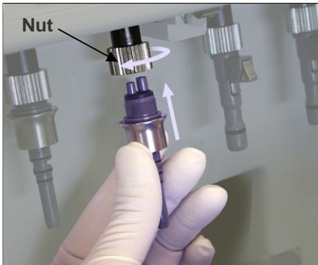
Fit the replacement coupling onto the nozzle and tighten up its nut.
