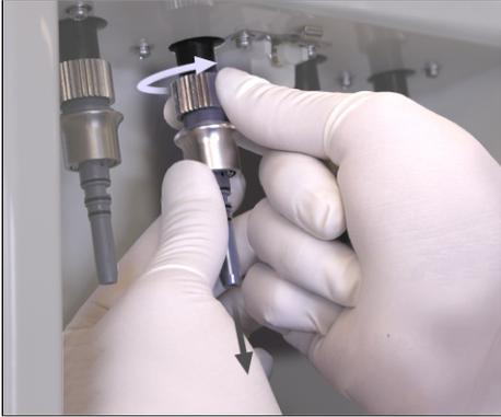
Loosen its nut and take the coupling off. Clean it with Ethanol for Disinfection (Ethanol 80 vol%).
