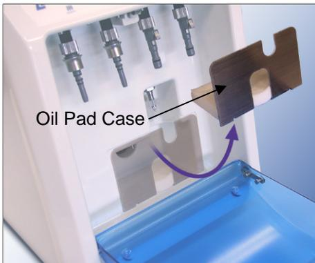
2. Take the pad out of the case and replace it with a new one.
