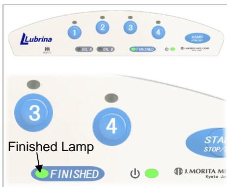
When the maintenance for all the handpieces is completed, their lamps will go out, a beep will sound and the Finished Lamp will light up.
