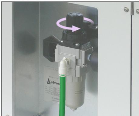
2. Put a container under the regulator and then press the drain valve.
