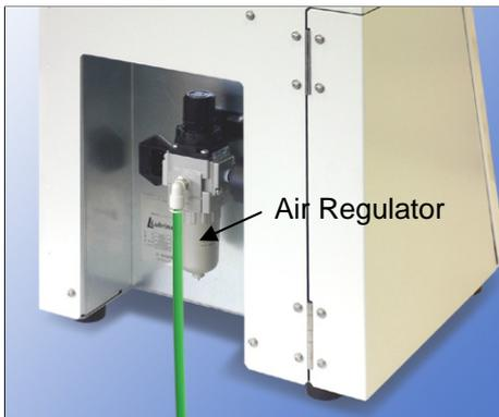
1. Turn the dial on the air regulator until the pressure drops to 0.
