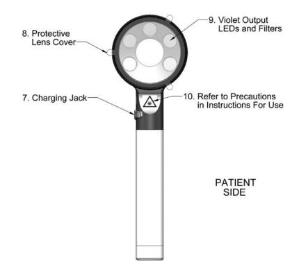
the 5 violet LEDs. Pressing the button a second time will turn off the 5 violet LEDs and the unit will return to standby mode. Once activated and after five minutes of continuous operation, the LEDs will automatically turn off and the unit will return to standby mode to conserve battery power. The Bio/Screen will operate for approximately 60 one-minute examinations starting with 100% charge.
