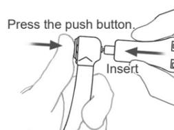
Press the push button firmly and insert the chuck grip tester straight at the same time.
