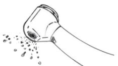
Connect the handpiece to its tube. Operate the handpiece for at least 15 seconds to expel excess oil from the head, and then wipe it off with a piece of gauze. Disconnect the handpiece from the tube.
