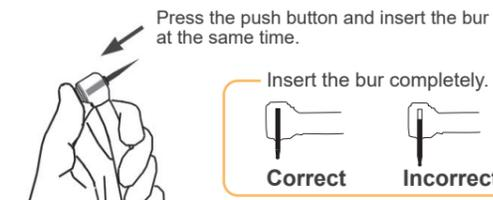
Press the push button firmly and insert the bur all the way in at the same time.
