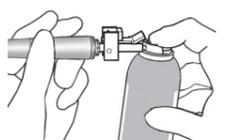
Insert the spray nozzle into the handpiece connection end, hold it firmly, and then spray for 2 seconds.
