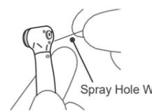
Clean the spray hole(s) with the spray hole wire provided, and rinse off the handpiece in running water.
