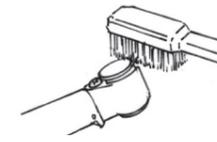
Clean the parts in running water with a toothbrush.
