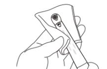
Wipe the whole handpiece with a piece of microfiber cloth (e.g., Toraysee for CE) that has been dampened with mikrozid AF liquid, FD322, or Rubbing alcohol.
