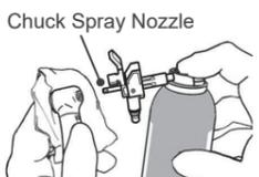
Cover the head of the handpiece with gauze, insert the chuck spray nozzle tip into the bur insertion hole, and then spray for 2 seconds.
