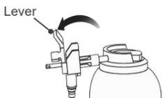
Push the lever on the spray nozzle up in the direction of the arrow.
