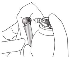
Shake the spray can 2 or 3 times before using it. Cover the head with a piece of gauze, insert the nozzle into the chuck and spray for 2 seconds.
