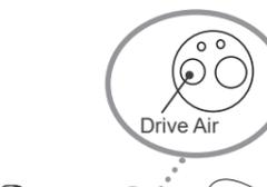
Insert the spray nozzle into the handpiece connection end for the drive air, hold the handpiece firmly and then spray for 2 seconds.
