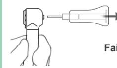
Chuck's gripping strength is weakened.
