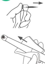
Remove the bur from the handpiece, turn on the water supply switch of the dental treatment unit, and run the handpiece for 20 seconds.
