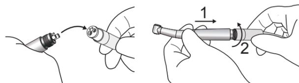
Line up the projections on the handpiece with the indentations in the tube and then tighten up the cover nut.
