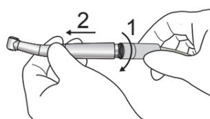
Hold the handpiece and unscrew the cover nut of the tube.
