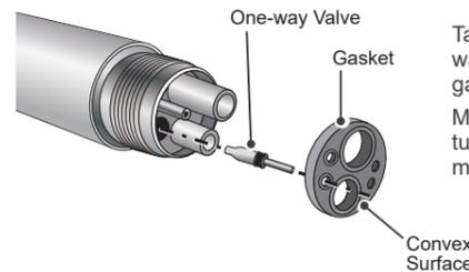
Take off the gasket with a needle. Take out the one-way valve. Slide a new valve into place. Put the gasket back on in its original position.
