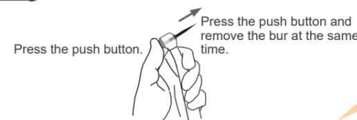
Hold down the push button firmly and pull the bur out straight.
