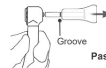
Chuck's gripping strength is normal.
