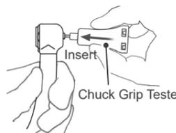
Insert the chuck tester straight in until it lightly touches the chuck mechanism.
