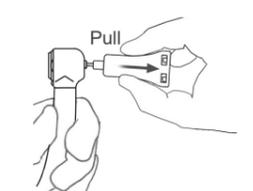
Pull the chuck grip tester slowly until the groove is visible.
