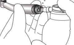
Connect the handpiece to its tube. Operate the handpiece for at least 15 seconds to expel excess oil from the head, and then wipe it off with a piece of gauze. Disconnect the handpiece from the tube.
