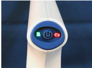
When battery is near end of charge, indicator turns RED
