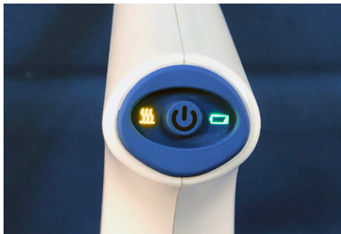
For the first minute of heating cycle, the temperature status blinks AMBER
