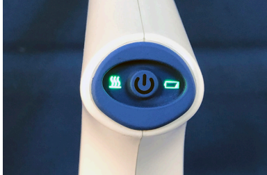
At one minute the temperature status blinks GREEN and at 2 minutes turns solid GREEN
