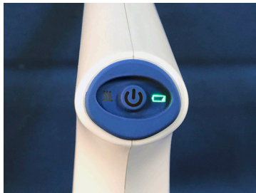
Turns GREEN when battery is completely charged
