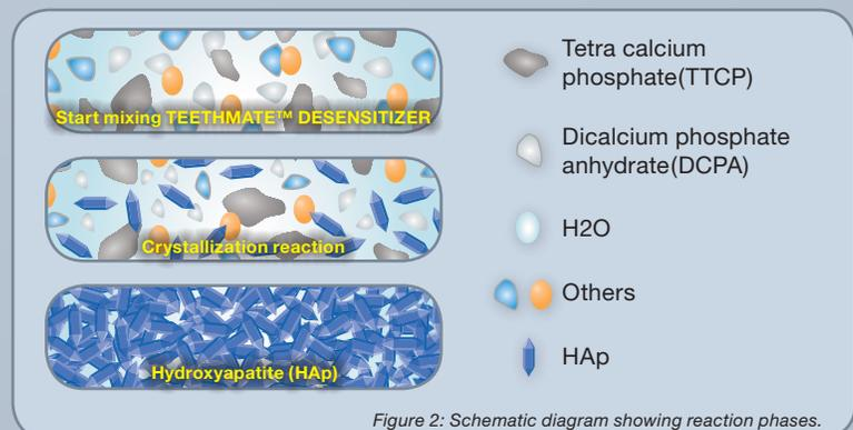
Figure 2: Schematic diagram showing reaction phases.
