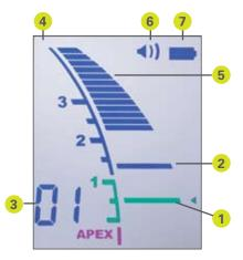
The color liquid crystal display is easy to read, providing a clear progressive display and high contrast. The positions of the Flash Bar and the Memory Bar can be set as guides for canal measurement and enlargement.
