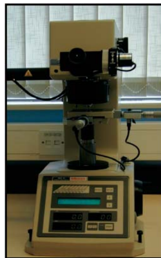
Photograph 2. Micro Vickers Hardness testing using the Mitutoyo MVK-H1.
