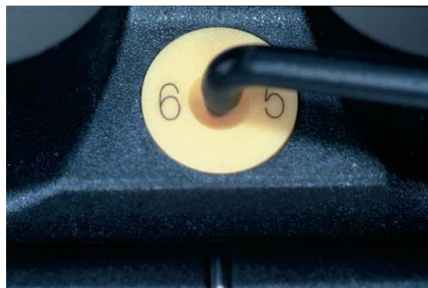
Figure 3: The ceramic standard is used for the periodical calibration.
