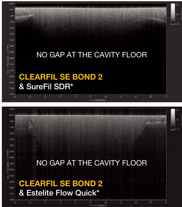
Fig. 7 Optical coherence tomography (OCT) images of the bonding interface with composite
